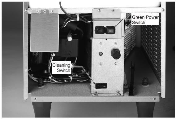
Front View With Front Panel Removed
