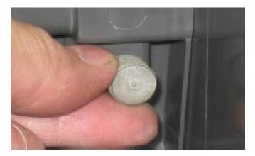
Remove Thumb Screw Holding Curtain
