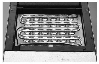
Pour Scale Remover Over The Evaporator Section
